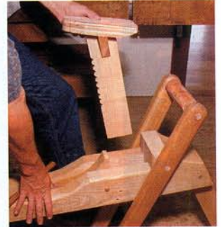
Cover both jaws with leather after assembly.
